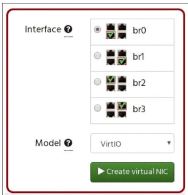
Figure 3: The first Ethernet interface found basically uses a bridge into which new VMs can plug.
