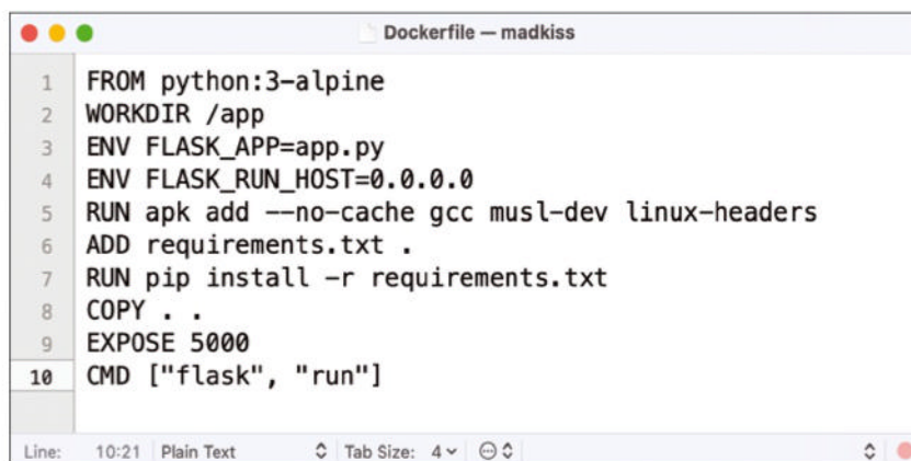
Figure 3: Without a Dockerfile, an Acornfile is useless. Acorn builds its own local container with docker build . To do this, you need a file named Dockerfile , and it must be syntactically correct.
